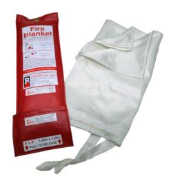
Made of Woven glass fibre. Totally asbestos - free. Certified to BS 476 Parts 4 (non-combustibility) and Part 7 (class 1 rating awarded for surface spread of flame). Able to withstand temperatures of up to 550°C. Use on fires involving flammable liquids and small fires in the kitchen. Effective against fires caused by oils, paints, spirits. Can be used to wrap around a person whose clothes are on fire and to wrap around the body while escaping.
